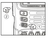
3. When you are satisfied with the Squelch threshold setting, press the **PTT** key momentarily to save the new setting and exit to normal operation.
